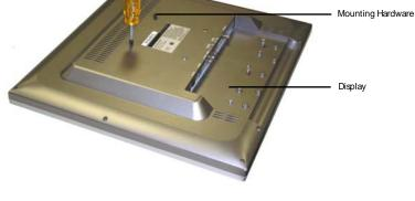
3. Lift the display and carefully guide the display with the two screws into the keyhole openings.
